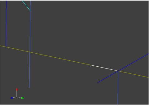
2. Choose Display |Beam Local Axis. The local axis shall be displayed for the selected element only. The axes color represents the axis name.
